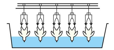
The electrical current, voltage, and duration must be validated and determined by the organization, taking into account the type, weight of the animal, and other variable factors.
